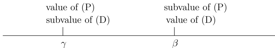
Figure 2.4: Gap between the values of the primal and the dual cone program.
